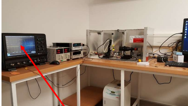
Transient Current Technique (TCT) set up. Detector signal is excited by picosecond pulsed laser and response waveform recorded by oscilloscope
